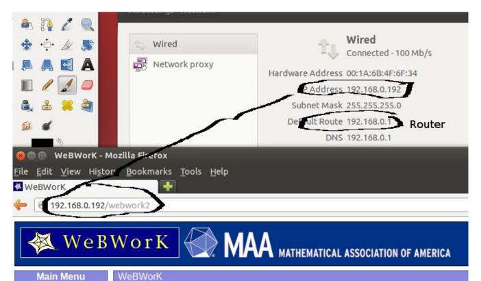
The top screen shows the relevant IP addresses for the local part of the network. The server is located at 192.168.0.192 and the router has an address of 192.168.0.1
